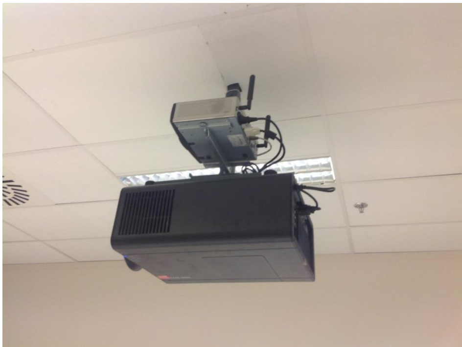
Figure 6: Example of correct ClickShare base unit installation
