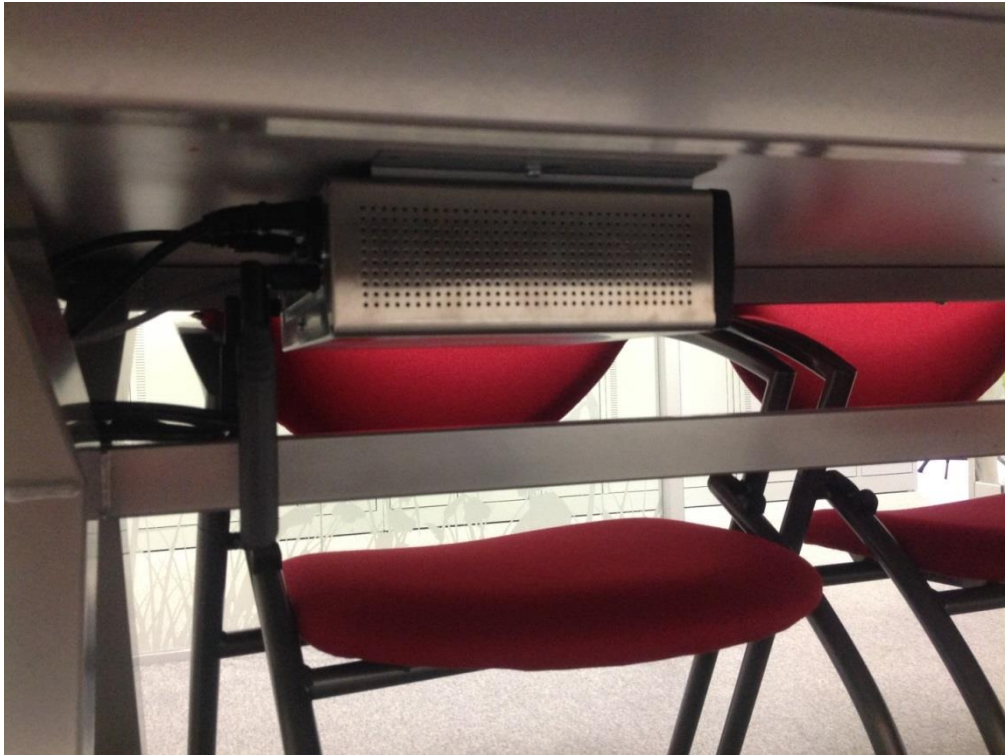
Figure 7: Example of correct ClickShare base unit installation
