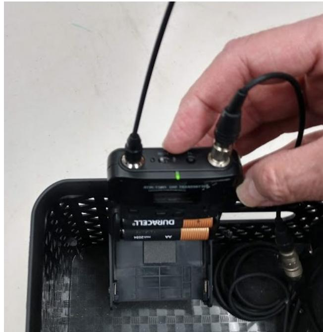
Body Pak with battery and control compartment open. Power switch (10) push up – ON position.
